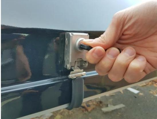
2. With one hand, push up the hard shell. The gas struts will allow it to open on its own.
