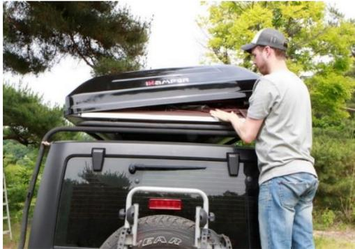
5. Pull down on the hard shell, and securely fasten the locks. Make sure the strap is tight by adjusting (twisting) the bottom U-shaped piece.
