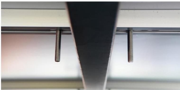
4. Take the bottom bracket **[A]** (with the round holes), and fit it under your cross bar so that the bolts go through it.
