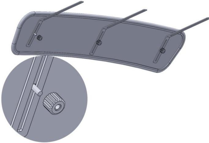
Take metal piece [C] and place the short side over bolt [F]. Then screw on head nut [G], and repeat for the other two bolts.
