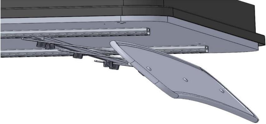
Adjust the height and position of the Wind Deflector by unscrewing the head nuts [G] and tightening them once the Wind Deflector is in the right position.
