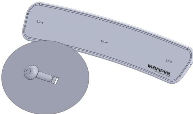
Insert 3 bolts [F] into the front of panel [A].
