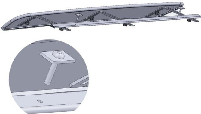
Insert the 2 bolts [H] in the holes on top of rail [D]. The wider sides (35mm) should be facing the front and back of the rail. Loosely screw on head nuts [G].
